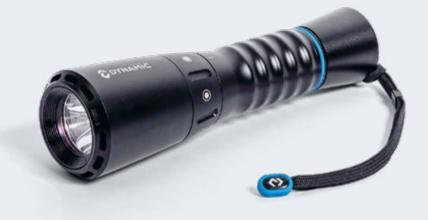
Dive light with a maximum power of 2000 lumens, a light angle of 15° and a colour temperature of 6500K. It has five output levels with a duration of: low 400 min, medium 250 min, high 200 min, strobe 500 min and SOS 200 min. Aluminum made; its weight under water is 215 grams (with battery) and 385 grams outside water (with battery). It has a length of 171.7 mm, a light head diameter of 49.5 mm and the light body diameter of 32 mm. It is waterproof up to 100 m deep.
