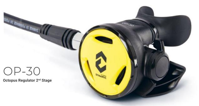
Adjustable Venturi to prevent freeflow on the surface and to reduce inhalation effort during the dive / Exhaust valve and deflector provide low exhalation work / LP hose tested for a maximum pressure of 34 bar / Mouthpiece made of high-end silicone / Yellow colour
